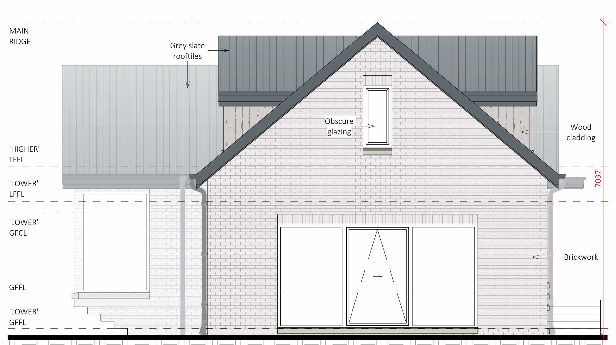
HOUSE TYPE 'C' - PROPOSED NORTH (SIDE-2) ELEVATION
