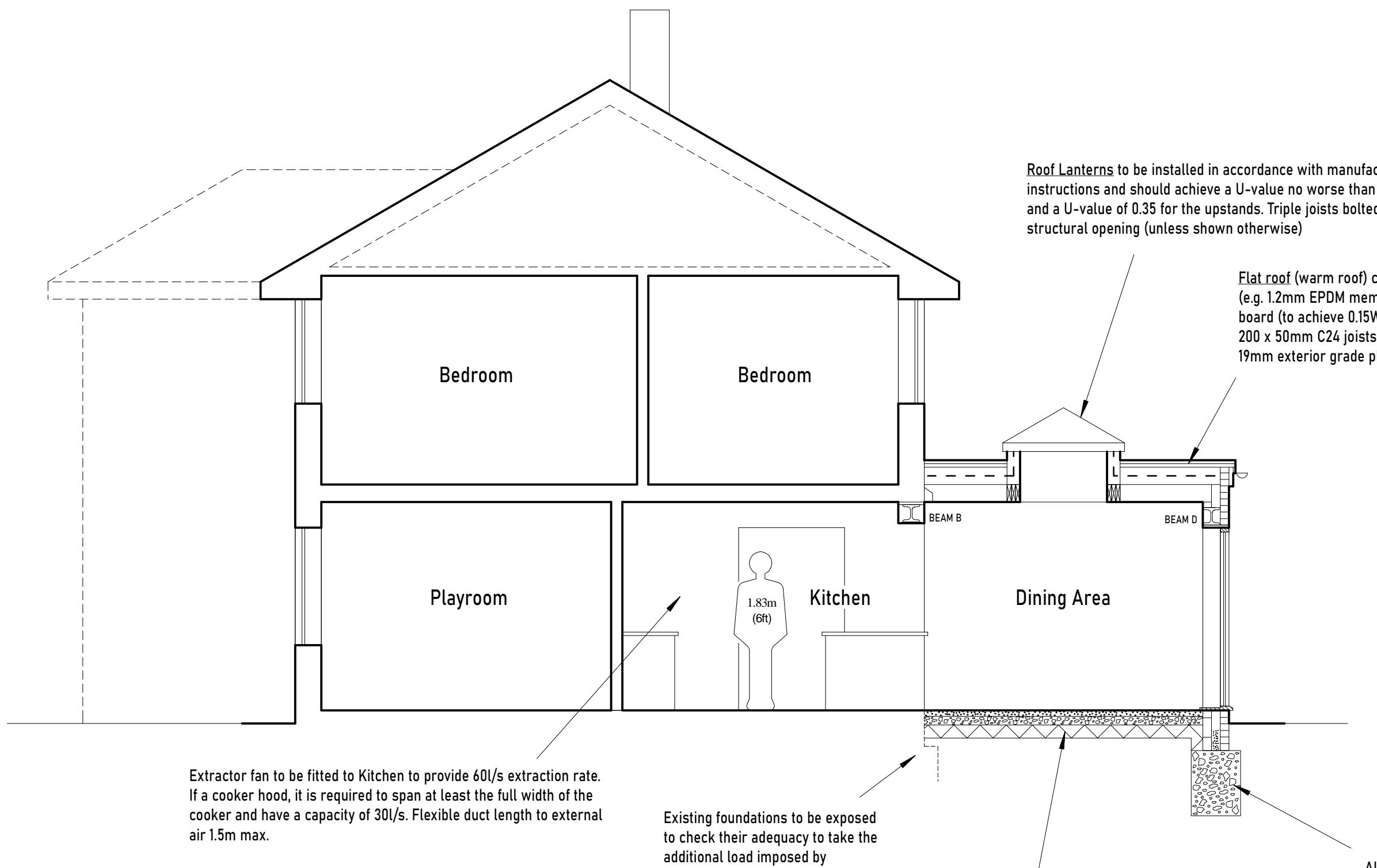
Extractor fan to be fitted to Kitchen to provide 60l/s extraction rate. If a cooker hood, it is required to span at least the full width of the cooker and have a capacity of 30l/s. Flexible duct length to external air 1.5m max.
