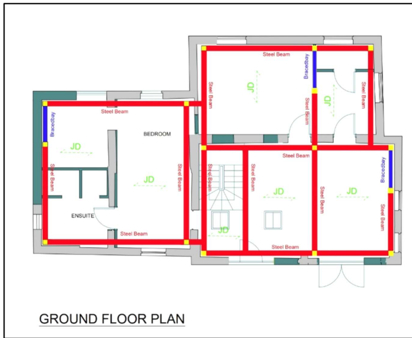
Photo 7 – Existing Cottage – Indicative Internal Structural Framing at Ground Floor Level.
