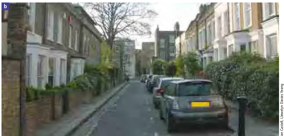
Figure 5.5 Two streets demonstrating different levels of enclosure. Street (a) has a height-to-width ratio of approximately 1:3, enabling a pleasant living environment to be shared with functionality in the form of traffic movement and on-street parking, some of it angled. Street (b) has a height-to-width ratio of about 1:1.5. Again, this works well in urban design terms, but the need to accommodate on-street parking has meant that traffic is restricted to one-way movement.
