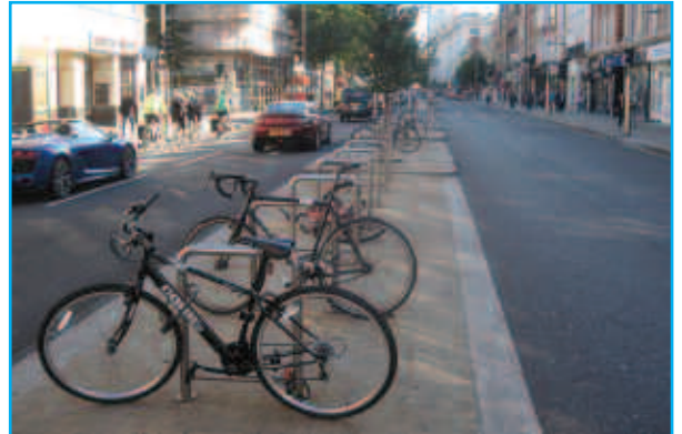
Cycle parking on central reservation, Kensington High Street. Generous spacing between the cycle racks enables pedestrians to cross between the parked cycles.
