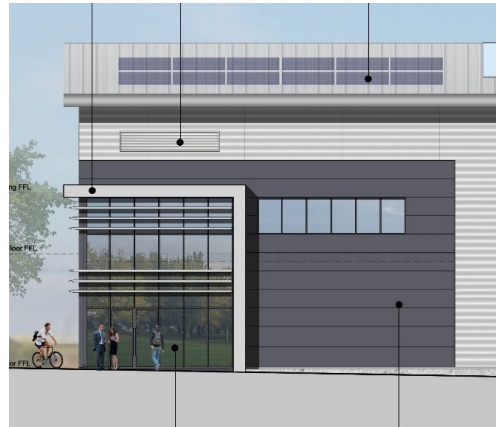
Dual aspect office fronting two elevations with fully glazed corner entrance & metal or timber bris soleil to south/west facing elevations
