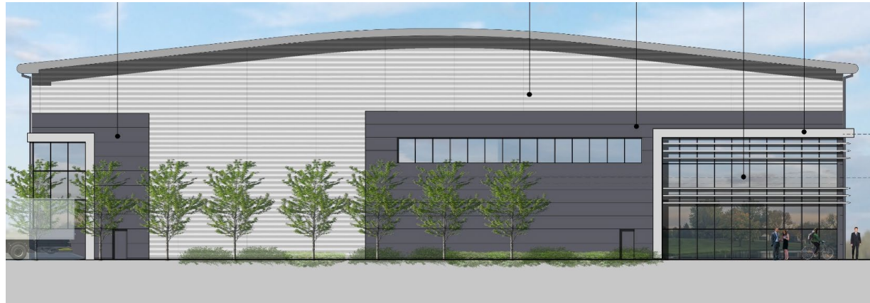
Dual aspect office fronting two elevations with fully glazed corner entrance & metal or timber bris soleil to south/west facing elevations
