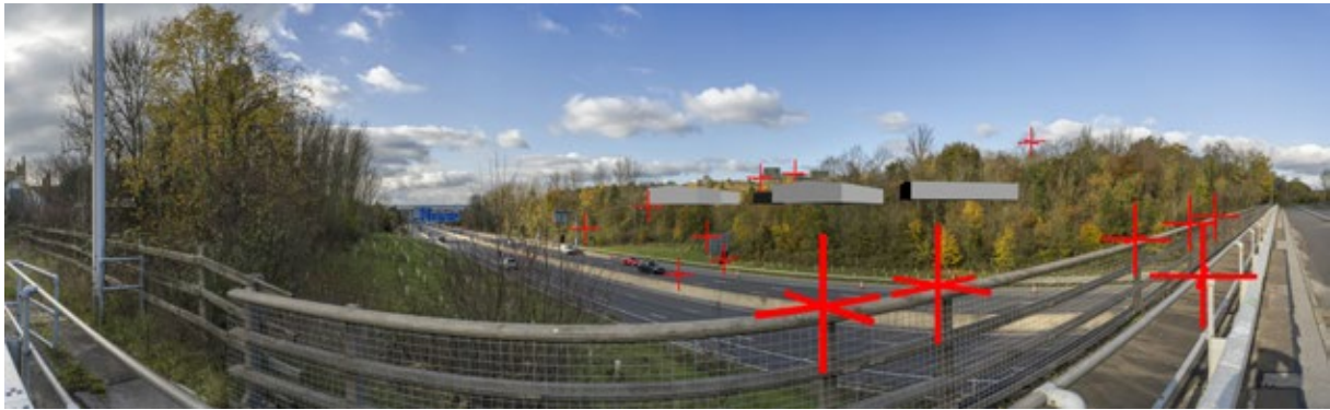
01.7 Screen grab of model matched to photograph
