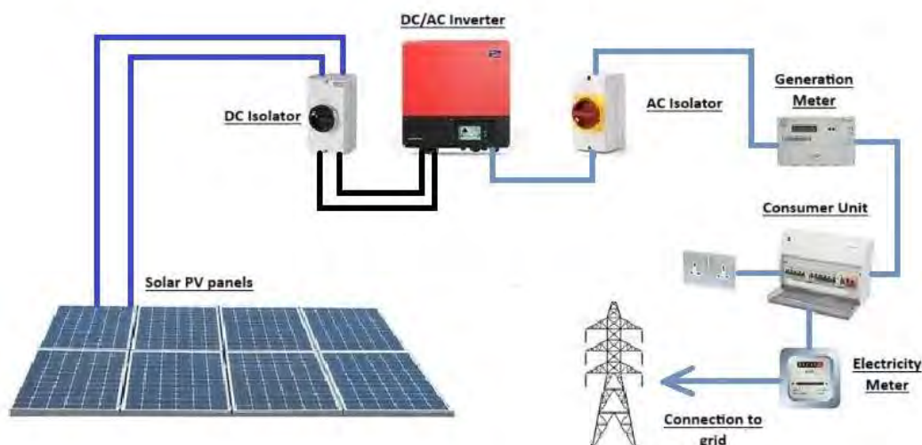
Figure 13 – Photovoltaic Panels – Typical Diagram
