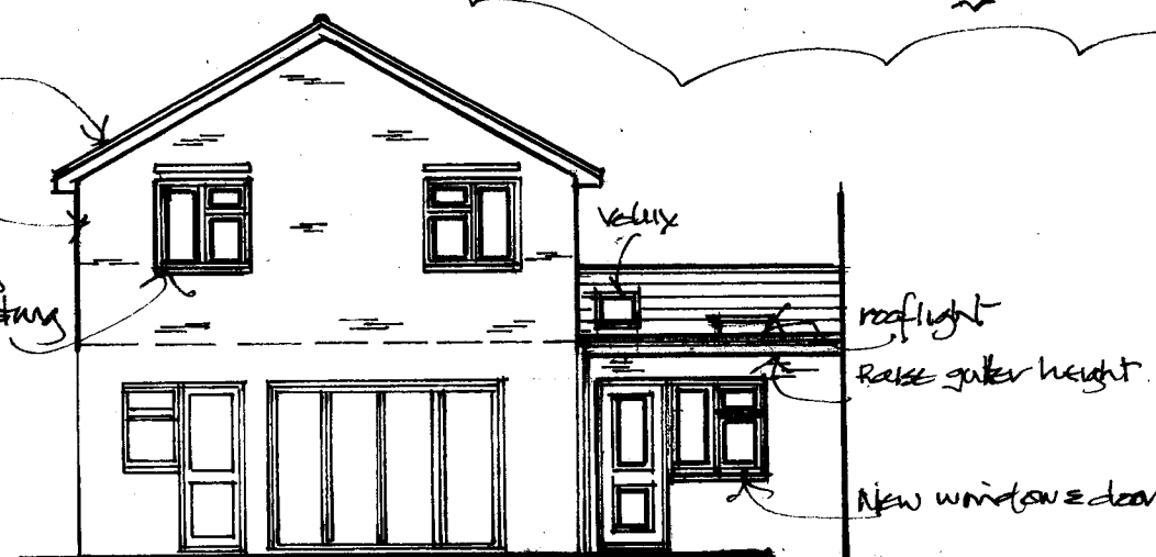
North West Elevation
