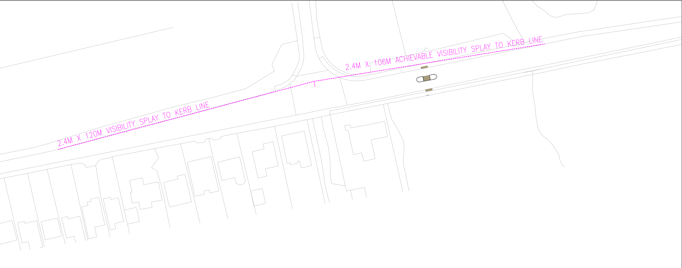
ACHIEVABLE VISIBILITY TO KERB LINE
