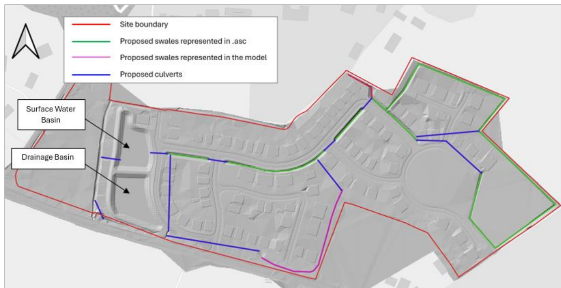
Figure 6-1: Post-development model schematic based on illustrative masterplan
