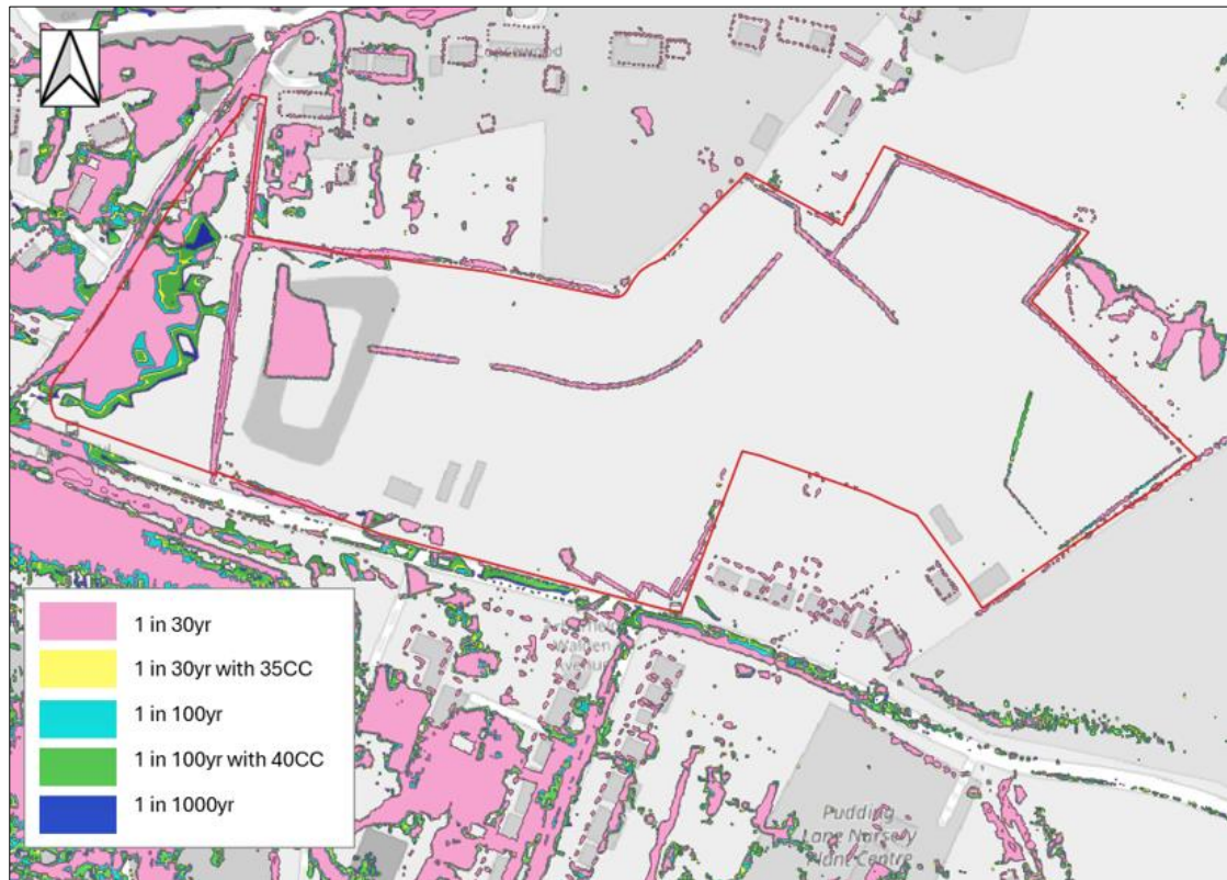
Figure 7-1: Post-development peak modelled flood extents
