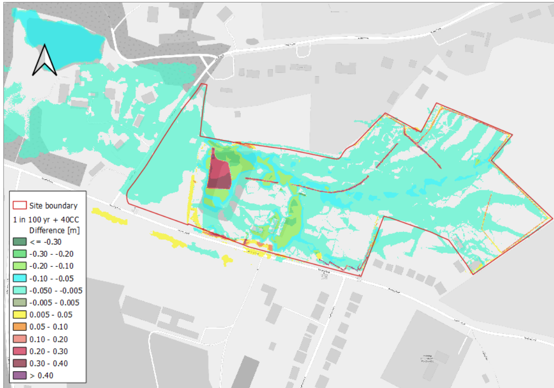
Figure 7-3: Change in peak flood depths – 1% AEP plus 45% climate change
