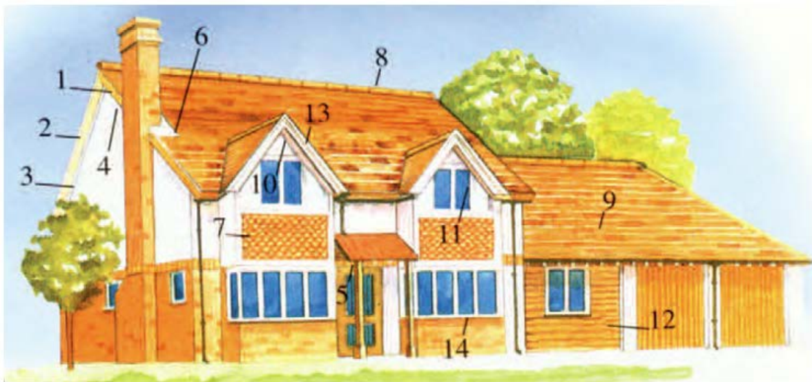
Building Features Commonly Used by Roosting Bats
