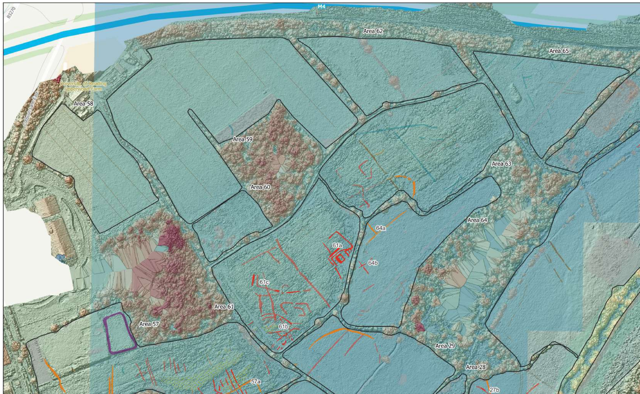
MSSU1348 - Loddon Garden Village, Reading Figure 37 - Combined Interpretation over 5cm Photogrammetric DSM and Hillshade (North-west). Hillshade Parameters: Azimuth 315° ; Angle 45° ; Z Factor 3.0 1:3,000 @ A3 Copyright Magnitude Surveys Ltd 2022 Contains Ordnance Survey data © Crown Copyright and database right 2022
