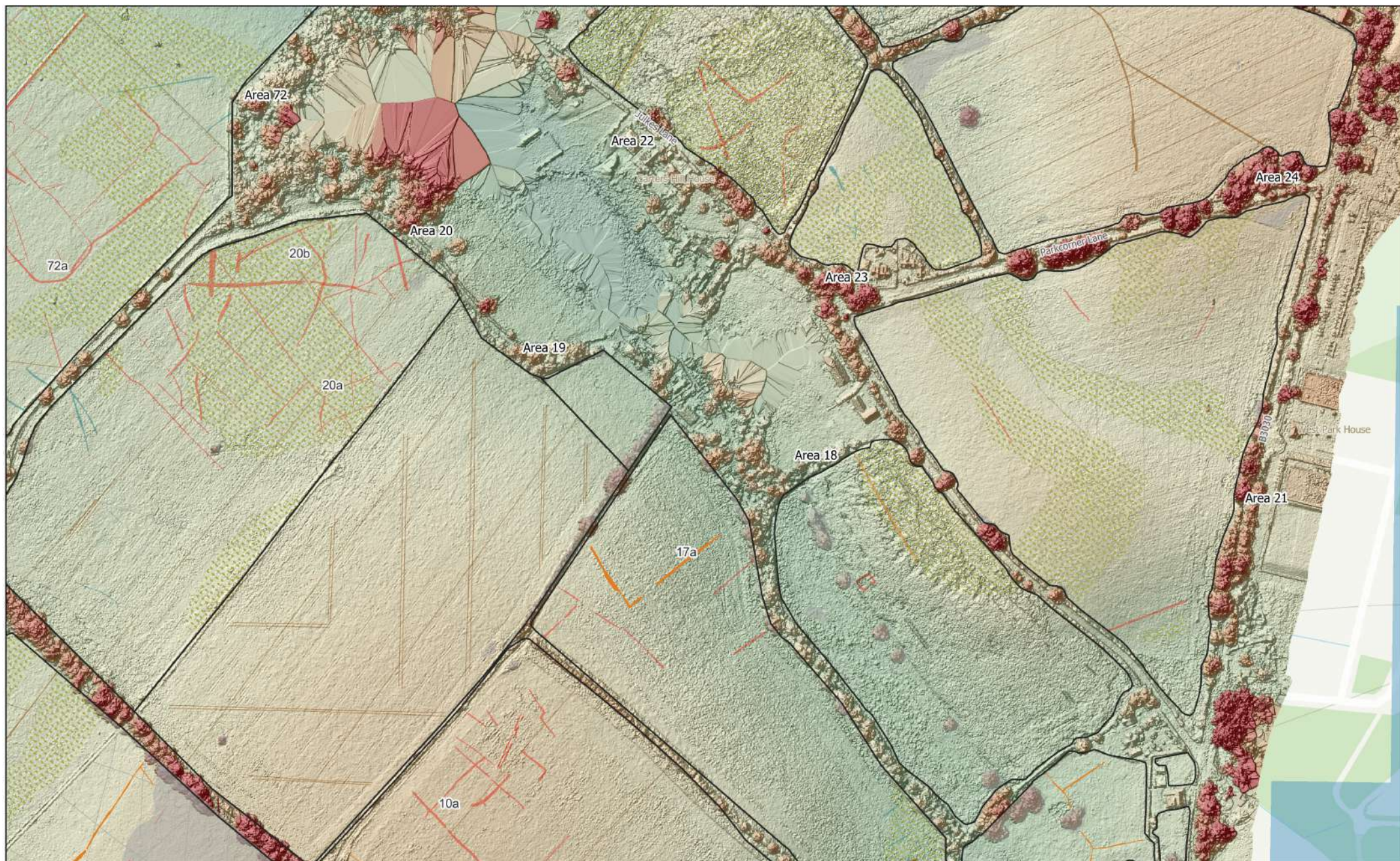
MSSU1348 - Loddon Garden Village, Reading Figure 17 - Combined Interpretation over 5cm Photogrammetric DSM and Hillshade (East). Hillshade Parameters: Azimuth 315° ; Angle 45° ; Z Factor 3.0 1:3,000 @ A3 Copyright Magnitude Surveys Ltd 2022 Contains Ordnance Survey data © Crown Copyright and database right 2022
