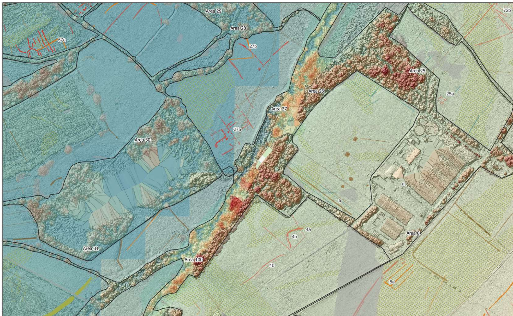
MSSU1348 - Loddon Garden Village, Reading Figure 22 - Combined Interpretation over 5cm Photogrammetric DSM and Hillshade (Central (South)). Hillshade Parameters: Azimuth 315° ; Angle 45° ; Z Factor 3.0 1:3,000 @ A3 Copyright Magnitude Surveys Ltd 2022 Contains Ordnance Survey data © Crown Copyright and database right 2022
