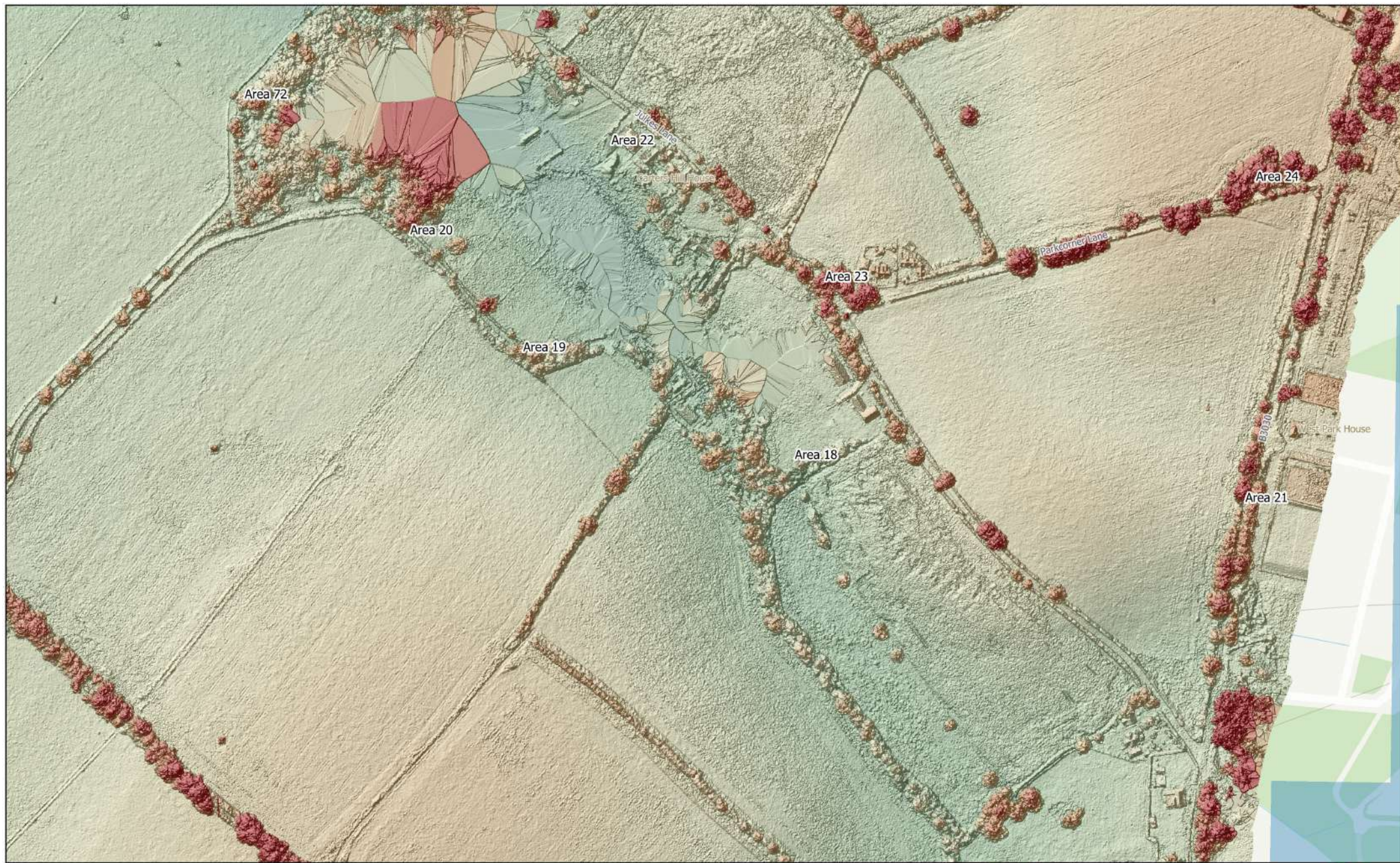
MSSU1348 - Loddon Garden Village, Reading Figure 14 - 5cm Photogrammetric DSM and Hillshade (East) Hillshade Parameters: Azimuth 315° ; Angle 45° ; Z Factor 3.0 1:3,000 @ A3 Copyright Magnitude Surveys Ltd 2022 Contains Ordnance Survey data © Crown Copyright and database right 2022
