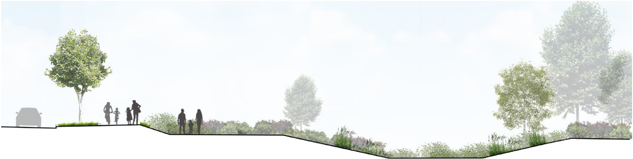
Illustrative section of occasionally wet area within drainage attenuation basin
