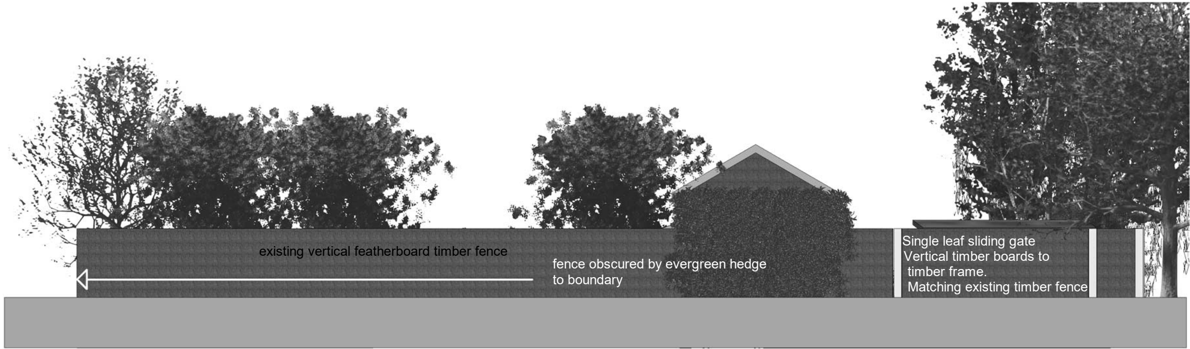
Elevation Northeast - after installation of gate
