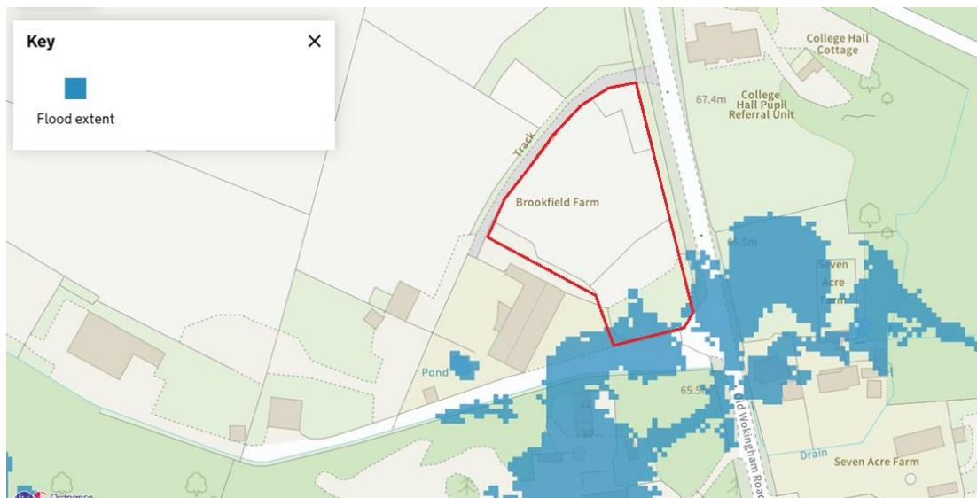
Approx red-line area showing part of the site is located in an area at risk of surface water flooding with an annual exceedance probability (AEP) of 3.3% (1 in 30) chance of flooding each year.
