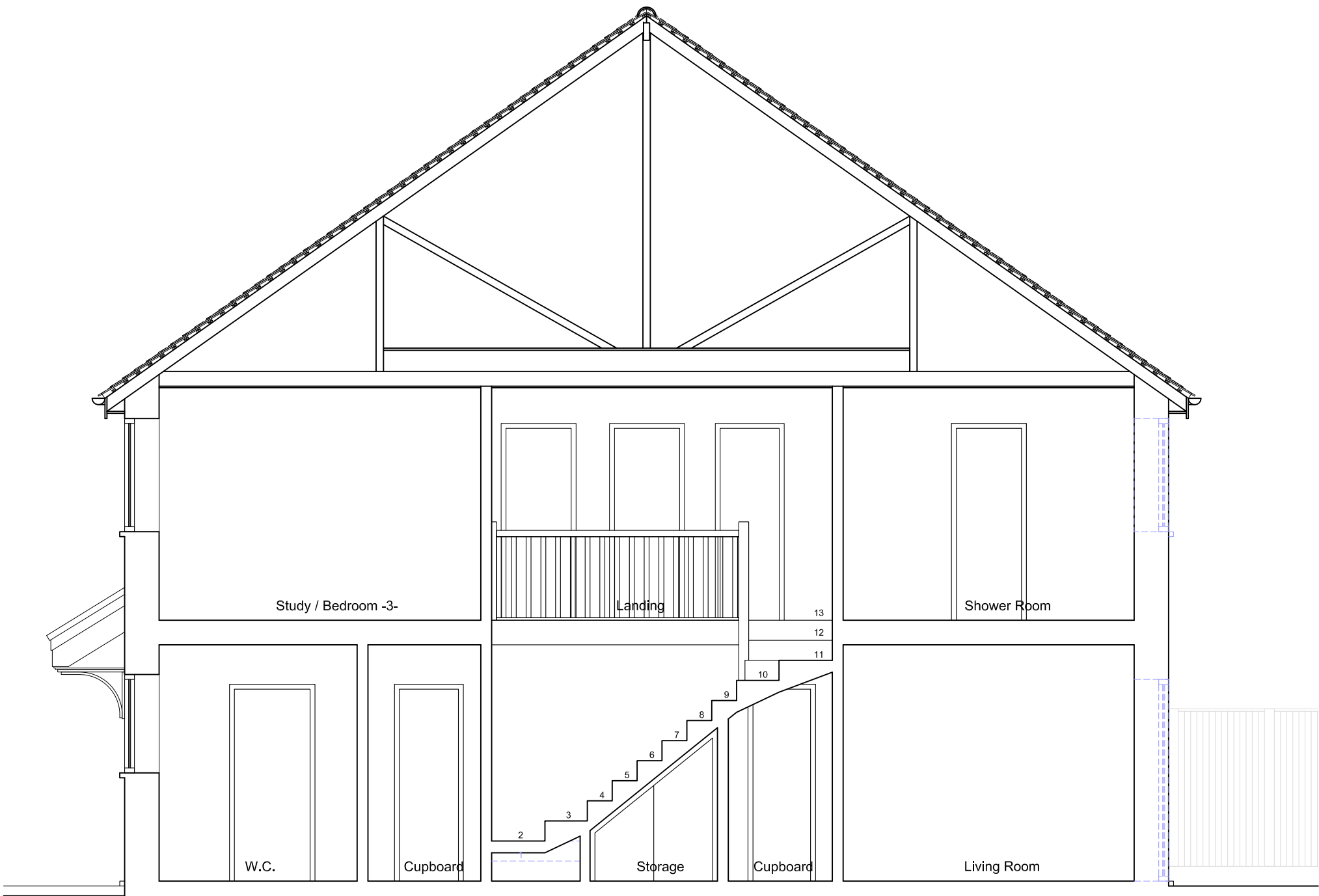
EXISTING SECTION A-A
