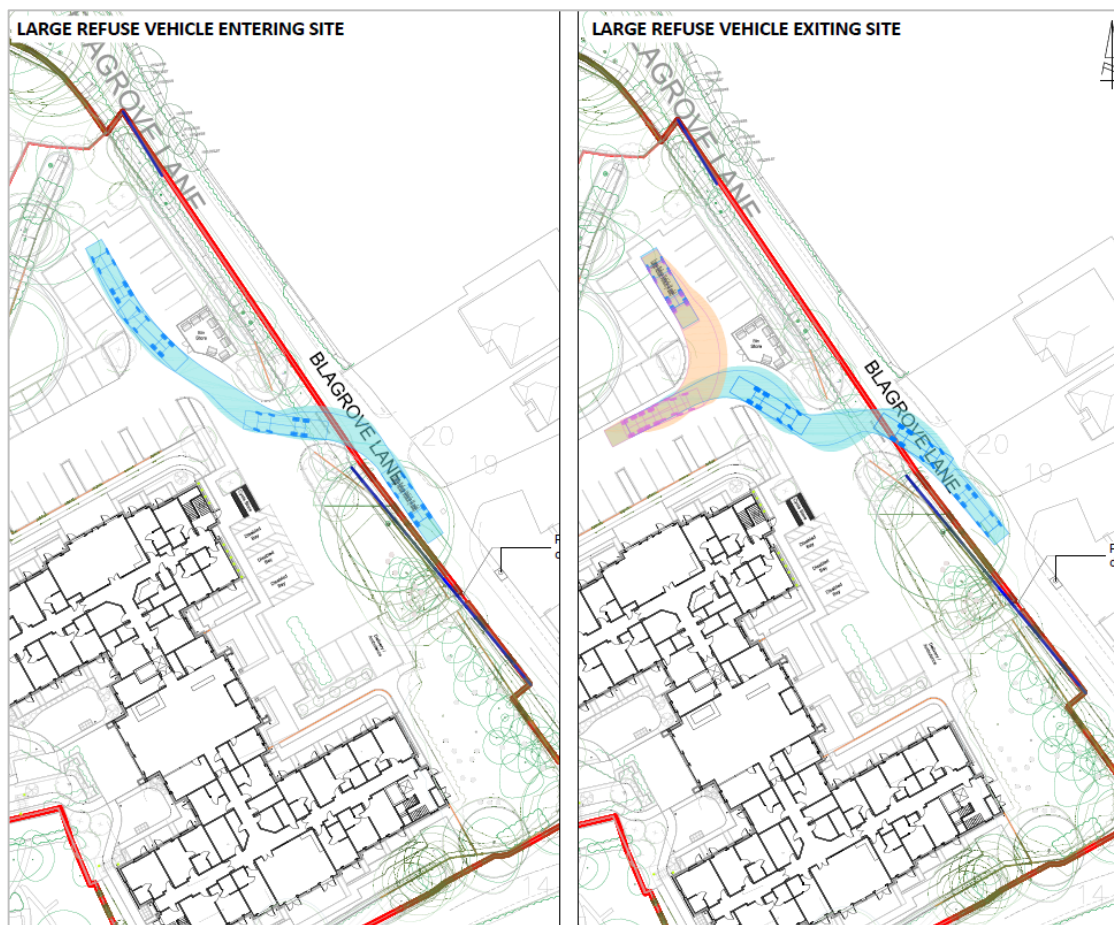
Image 3.3: Swept Path Analysis – Refuse Vehicle
