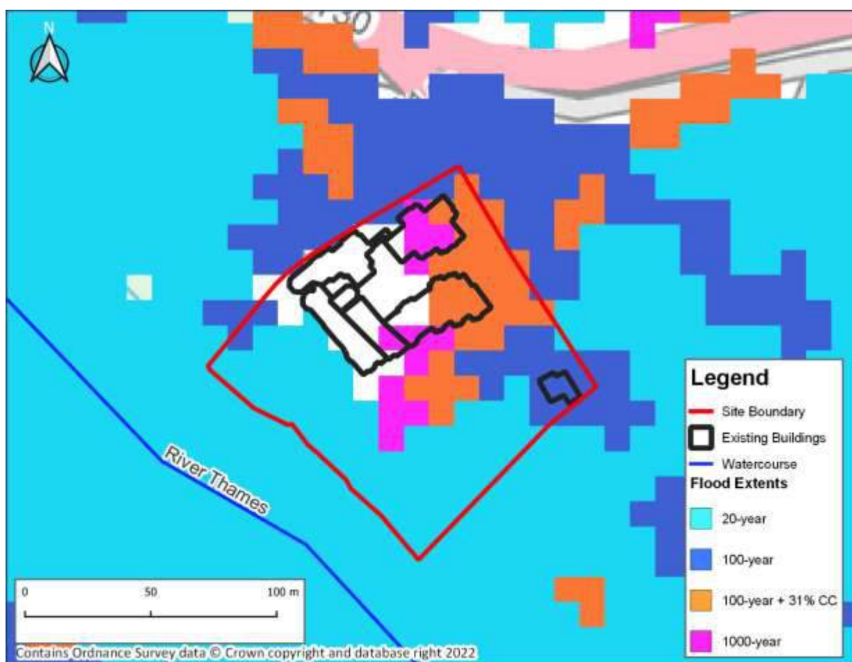
Figure 0-1: Baseline fluvial flood extents
