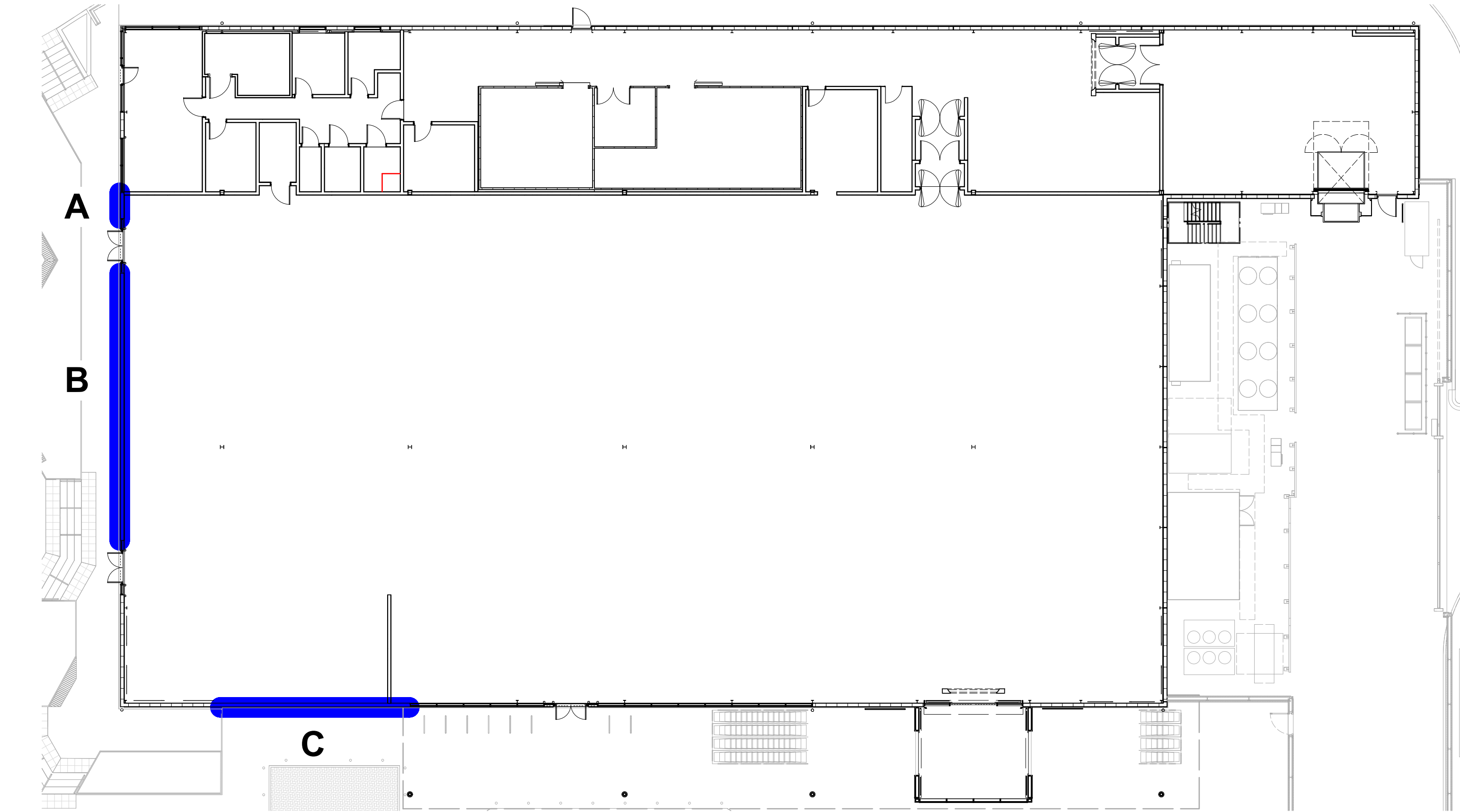
P Brickwork Feature Location Plan 1 : 200
