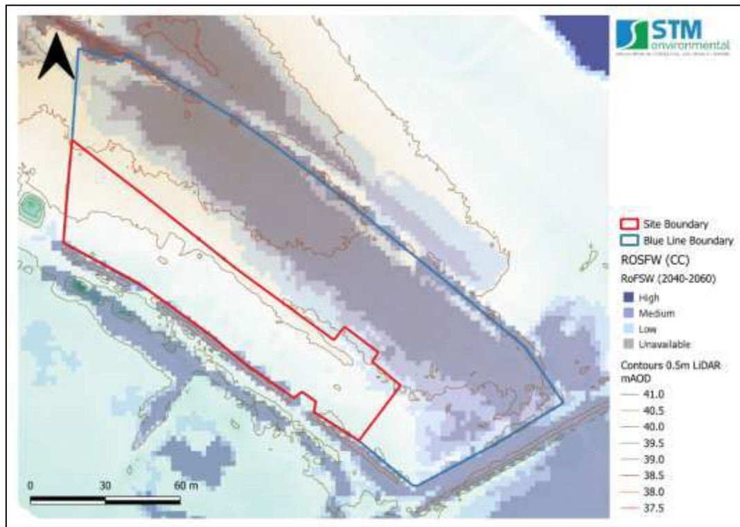
Figure 4: Surface Water Flooding Risk Overview
