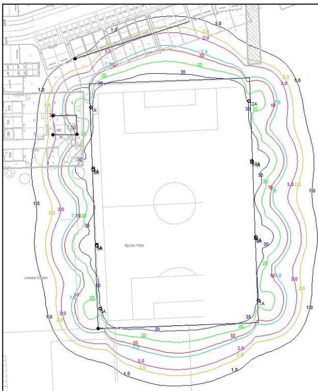
Figure 4.4 Horizontal Lighting Contour Plan at 0m Elevation
