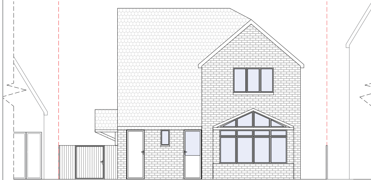
Existing North Elevation
