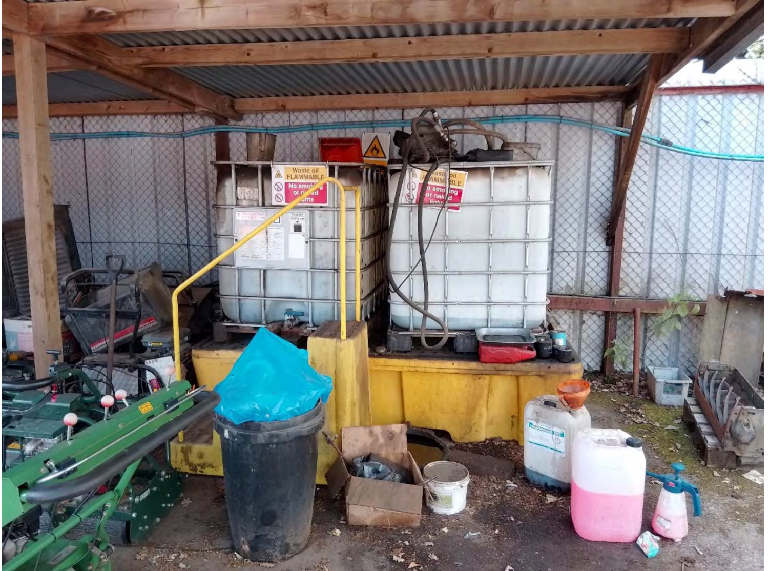
View of two vehicle oil IBCs sited atop plastic bunds in the southwest of the site looking southwest. Further miscellaneous items and open containers are stored in the vicinity. Moderate staining was observed around this area. Surface covering is poured concrete.
