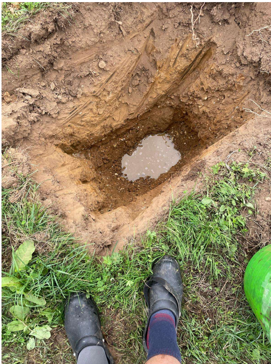
Photograph 2 - Trial excavation and small infiltration test hole during the falling-head test. The water shown was introduced for the test and is not evidence of groundwater.
