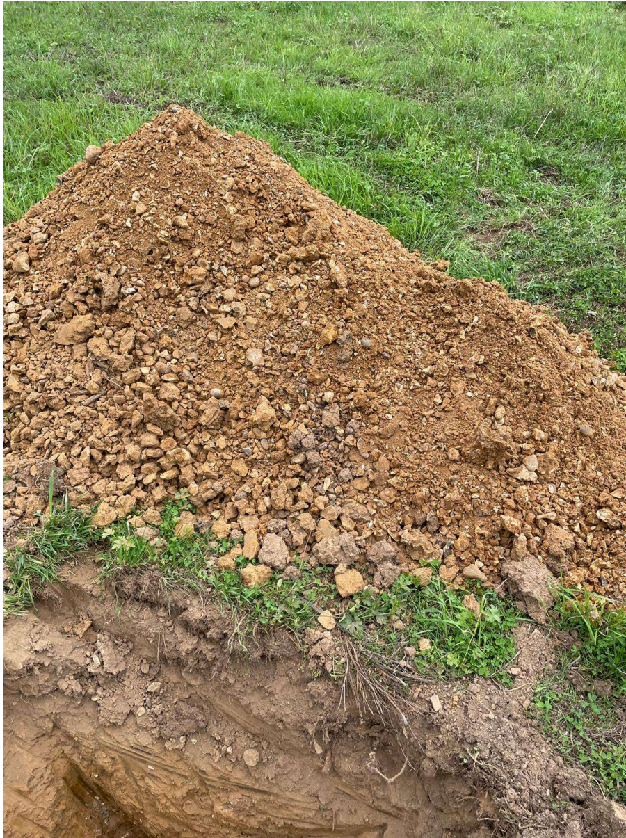
Photograph 1 - Excavated arisings from the trial pit showing significant gravel content encountered beneath the upper clay.
