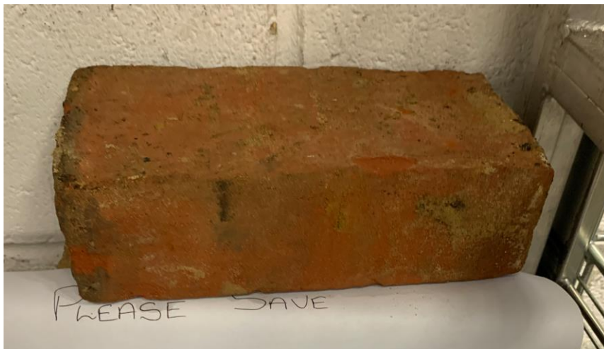
Figure 4. Photograph of type of replacement brick sourced from the reclamation yard.
