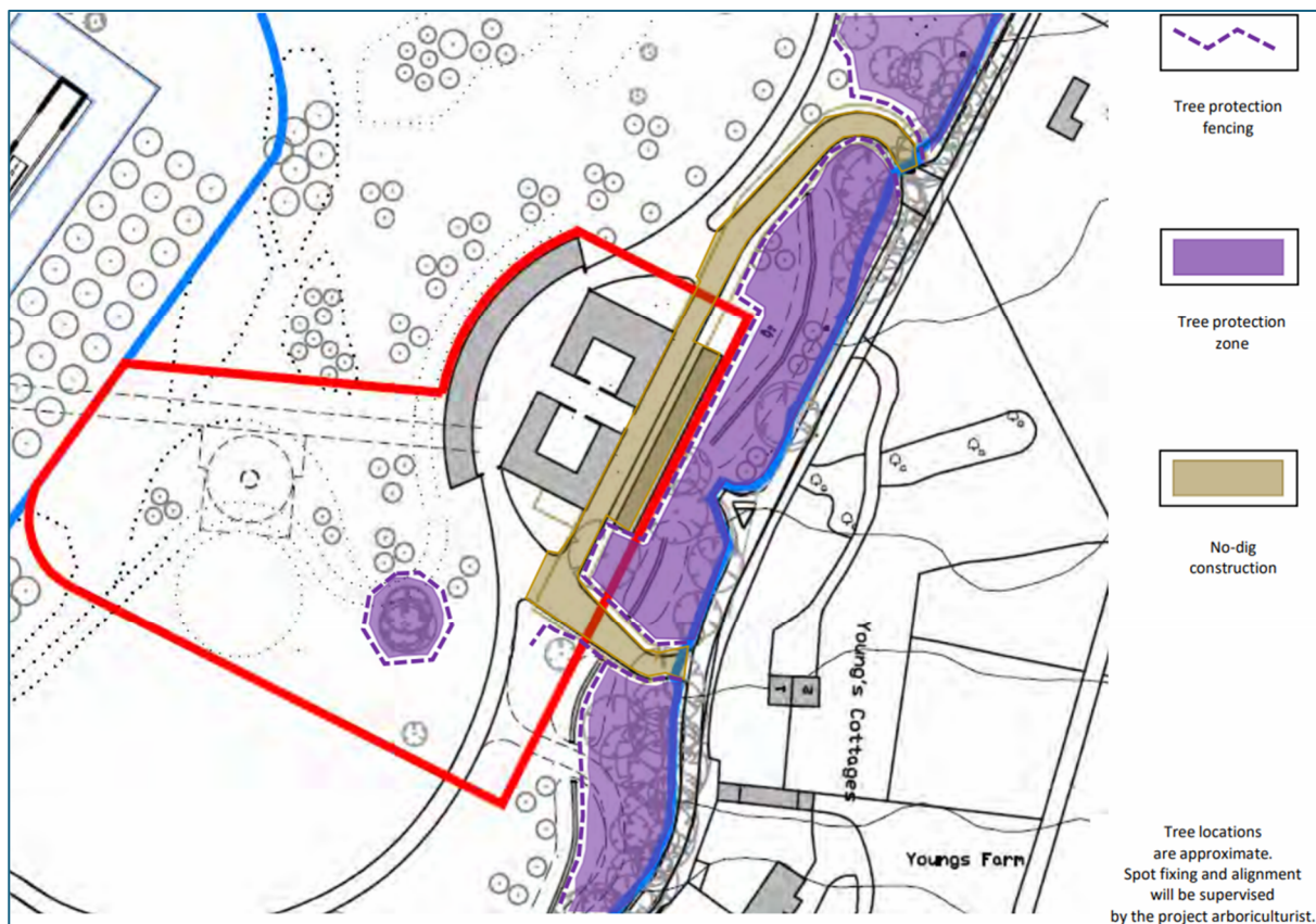
Fig 1. Revised protection measures around retained trees
