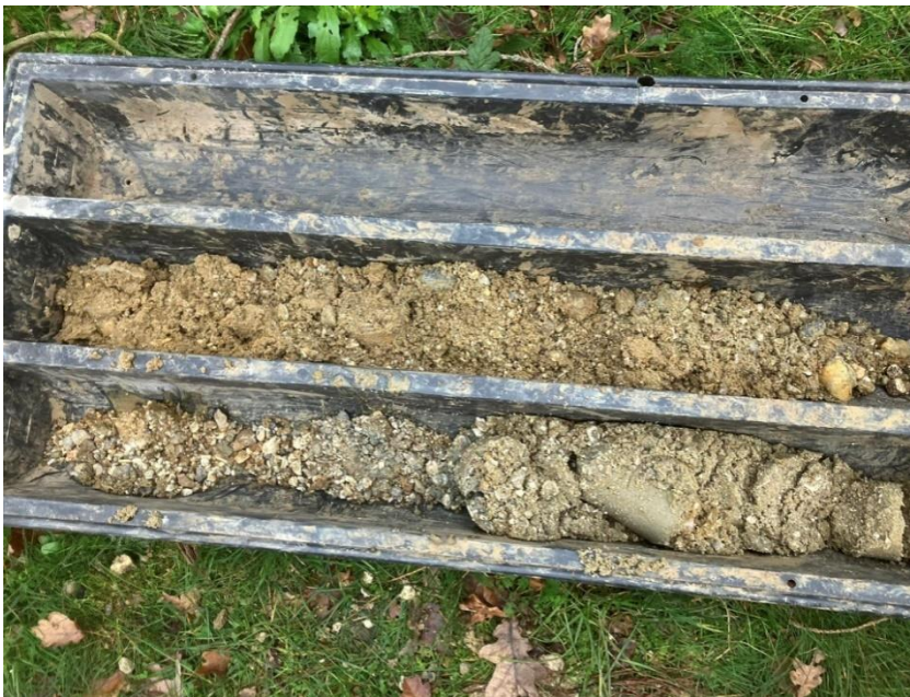
Photo 5 – BH1 Cores (3.00m – 5.00m)
