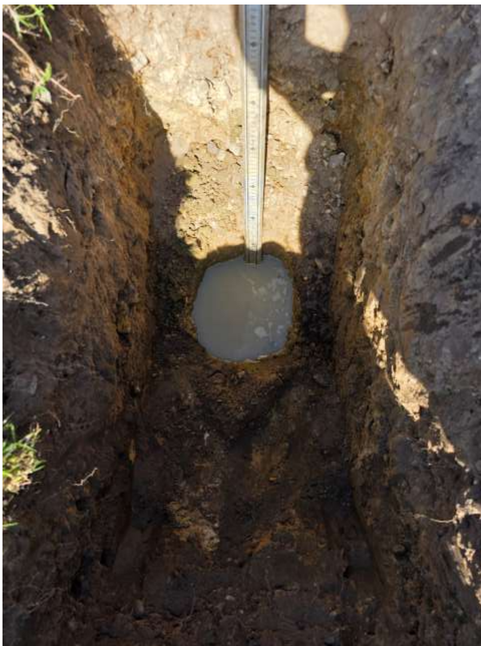
Figure 4 – SW1 during filling
