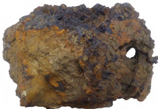
4, Slag with hole left by a tool used to remove the slag from the furnace, from layer 12315
