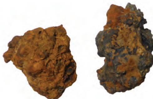
2, Magnetic slag and vitrified furnace lining, from pit fill 433
