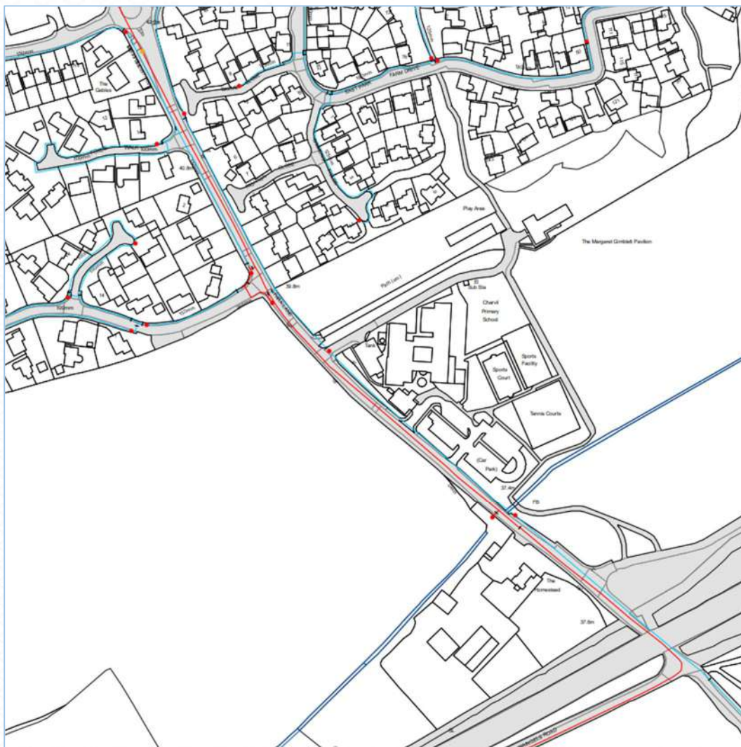
Figure 2.2: Thames Water Sewer Records
