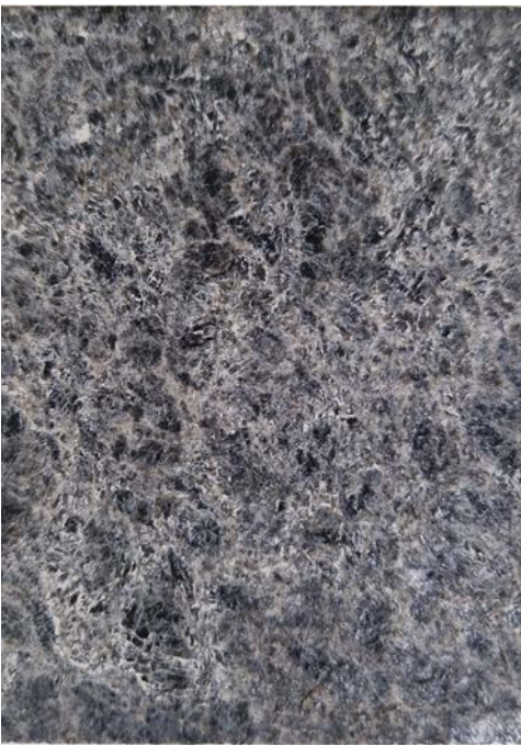
P02 (Q25/140) Granite sett paving Flamed finish. Colours: Angola Black, Fernando Roriz, Preta Odivelas, Silva Preta Flavaco
