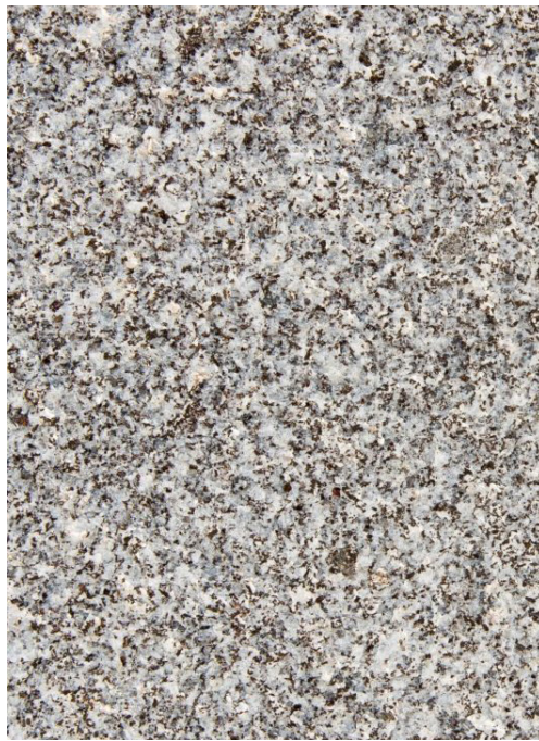
W01, W02 and W04 (Q10/121) Stone copings Finish: Bush hammered. Colour: Fernando Roriz Supplier: Hardscape Products or similar
