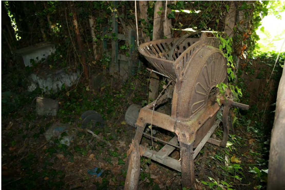
Detail of the hand driven Wrekin root (mangel) cutter. These are MC20th.
