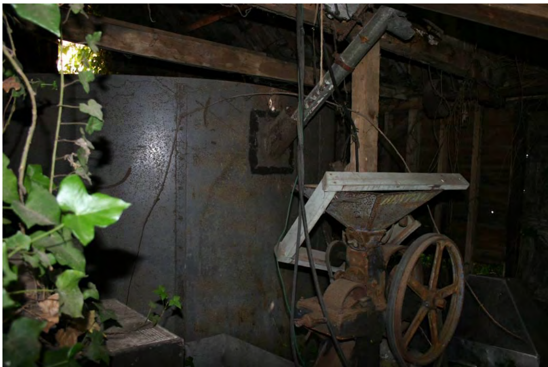
The grain silo and a Bentall's crusher grinder.
