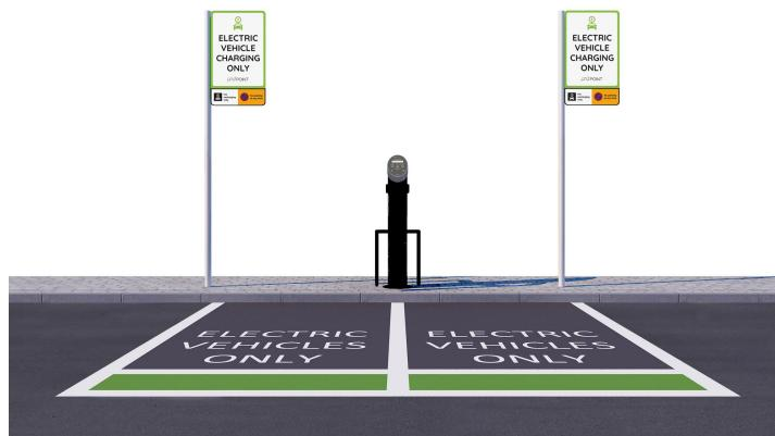
The Twin Charger, its signage, or charging cables when in use, should not obstruct the pavement. Under no circumstances should the width of a public footway be restricted to less than 1.2m, to allow suitable access for wheelchair users.
