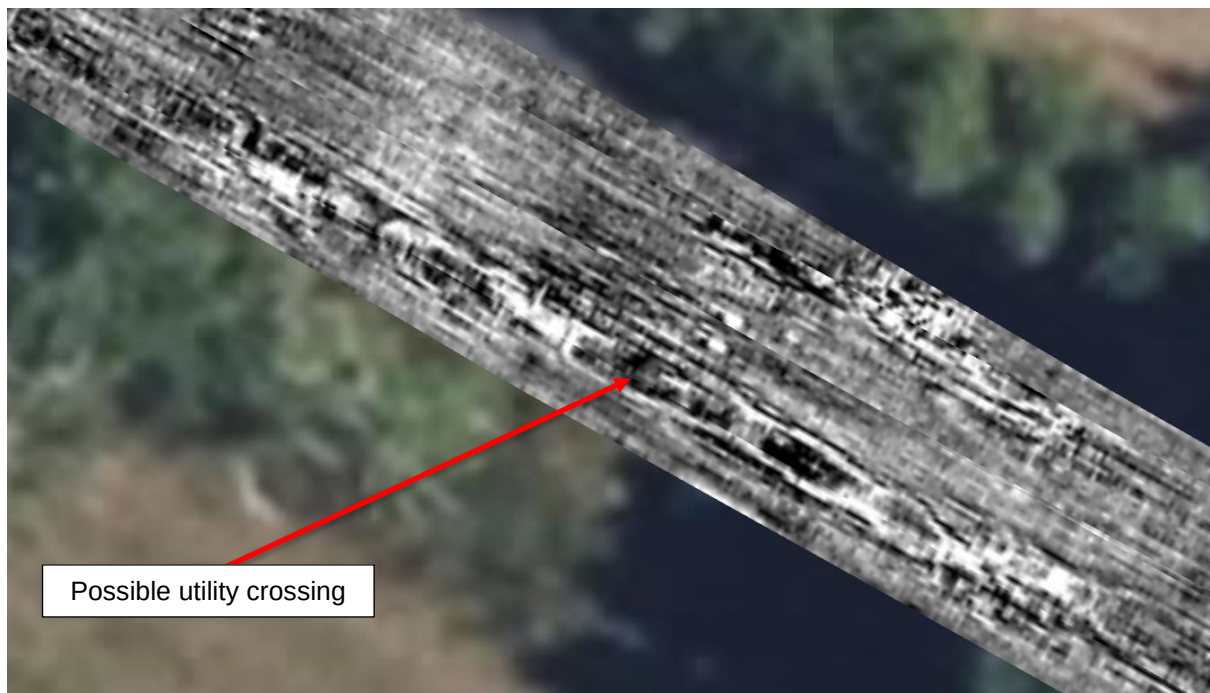
Figure 6 - Timeslice view (horizontal cross section) of suspected utility duct.
