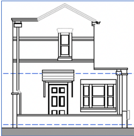
Image 3B - As-built upper banding on floor now wraps around the dwelling.
