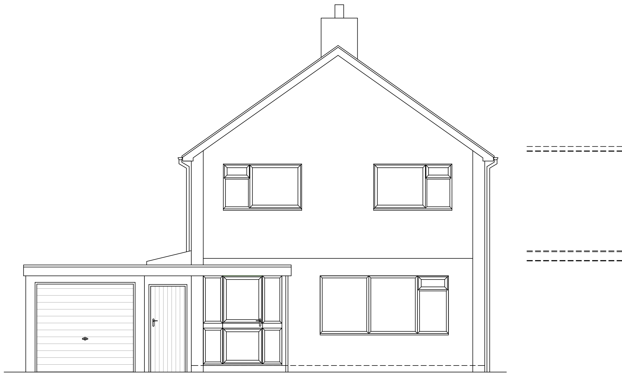
Existing front elevation
