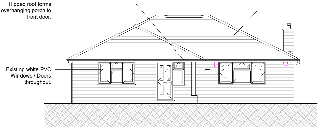
EXISTING WEST (FRONT) ELEVATION, 1:100
