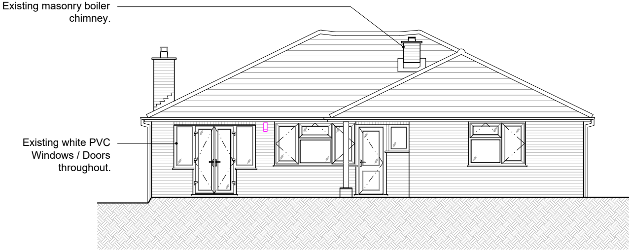
EXISTING EAST (REAR) ELEVATION, 1:100
