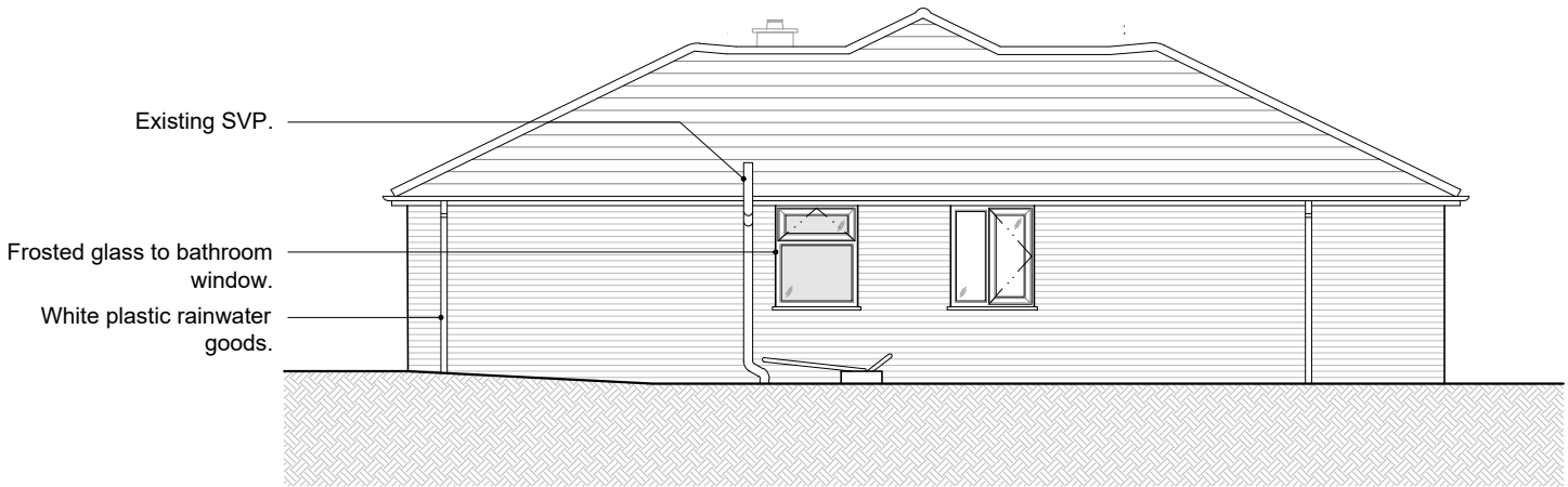
EXISTING NORTH ELEVATION, 1:100
