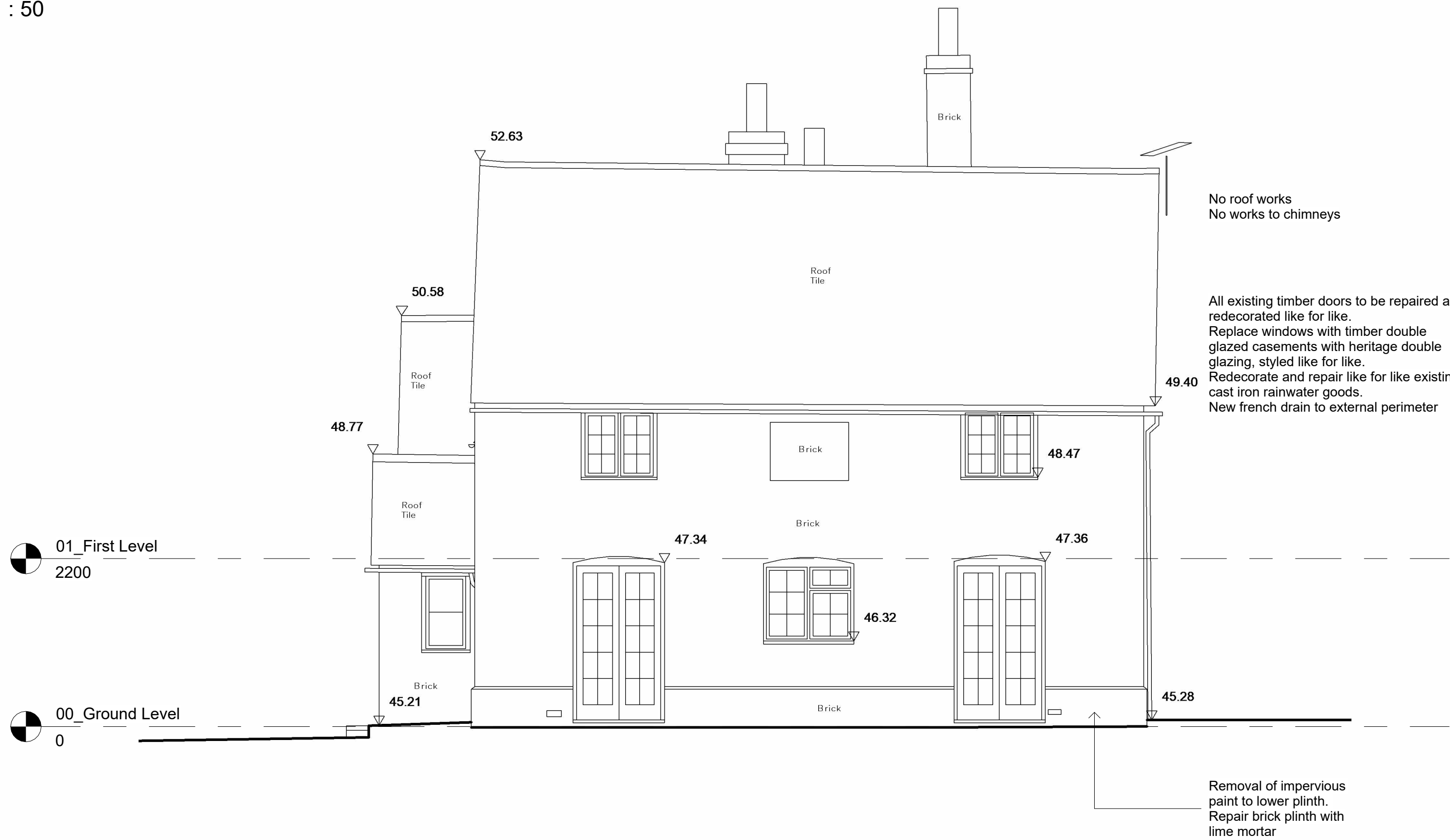
Proposed Farmhouse South Elevation 1 : 50
