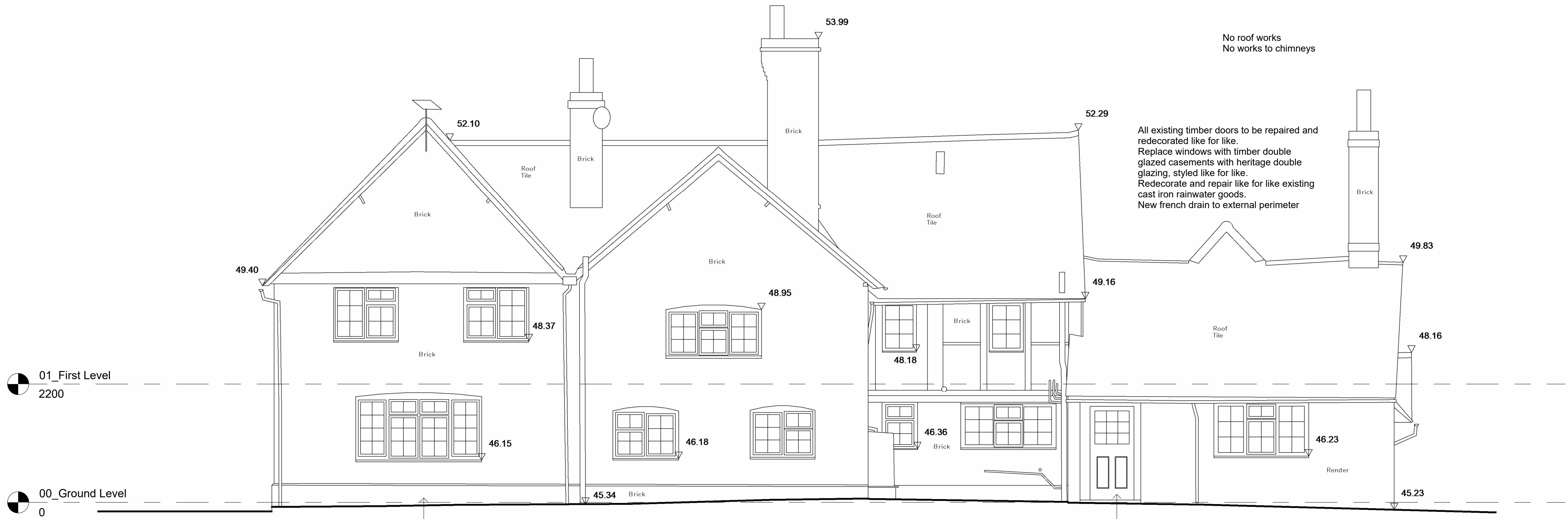
Proposed Farmhouse East Elevation 1 : 50
