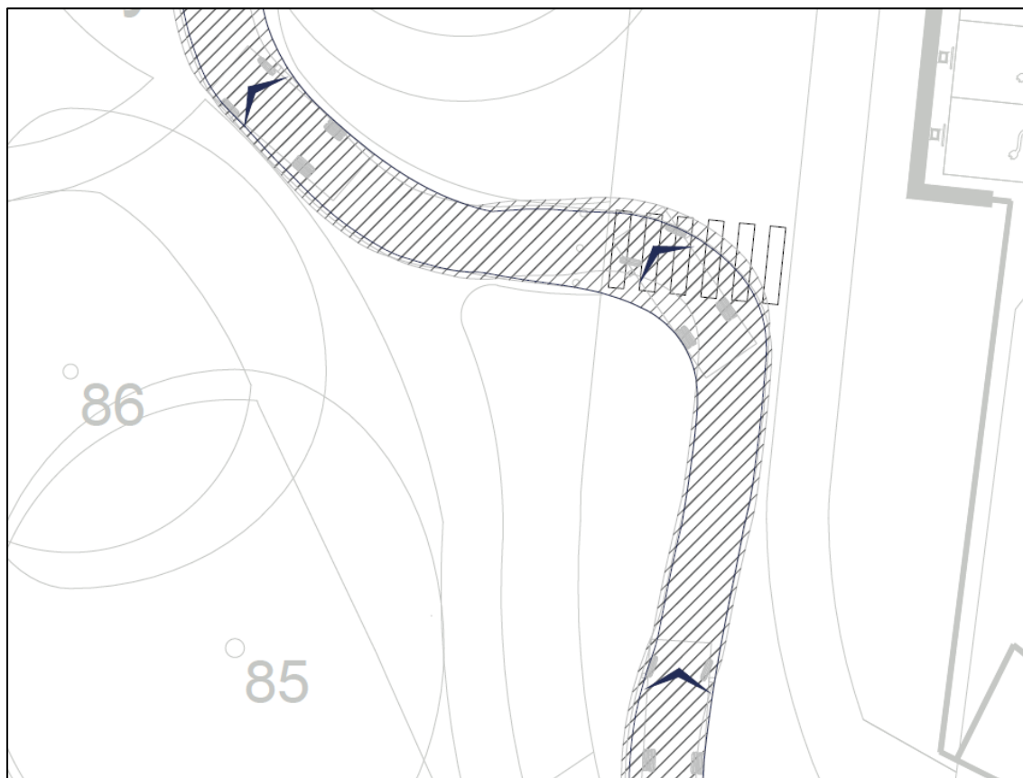
Figure 5 Panel Van Entering Amenity Area
