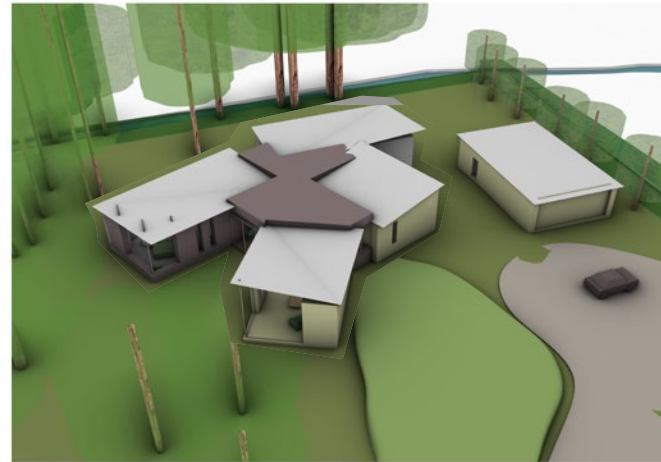
Central roof raised above
