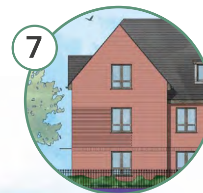
Linear brick detailing
