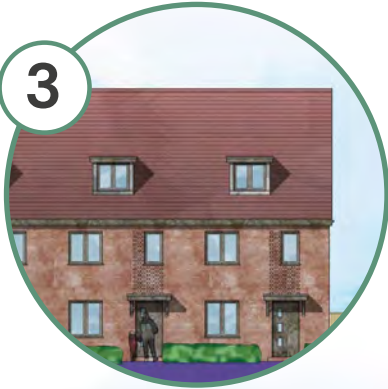
Extruded flemish brick detailing
