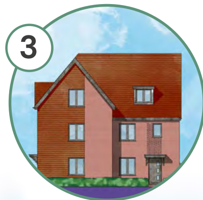
Contemporary use of tile hanging
