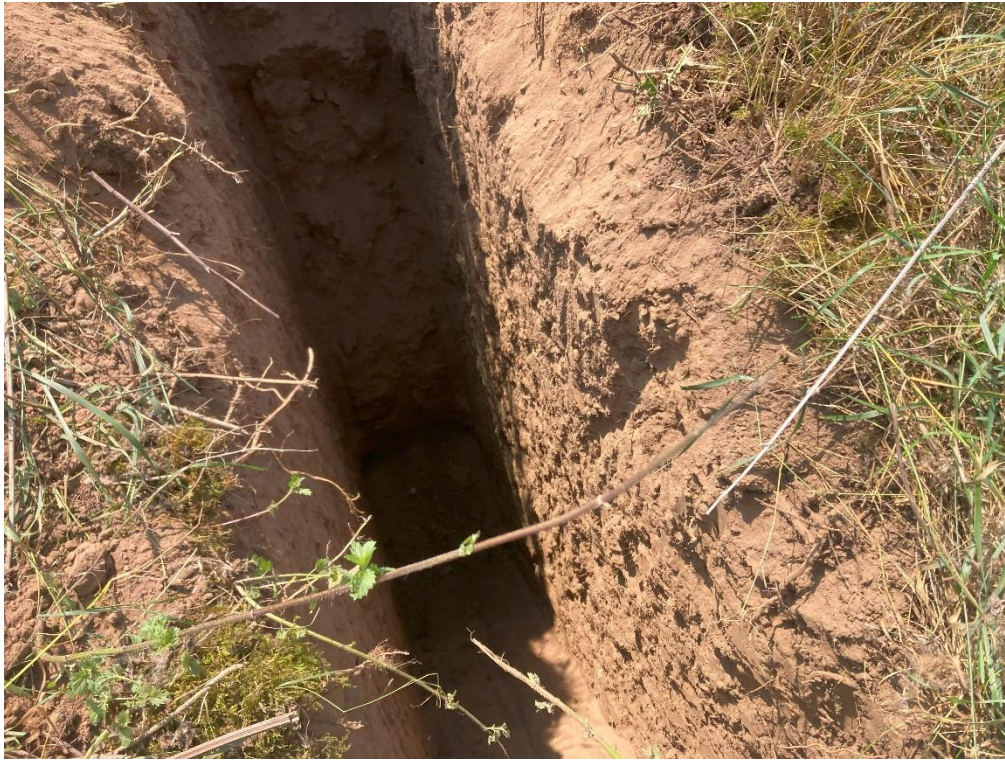
TP2 (Reworked Topsoil)
