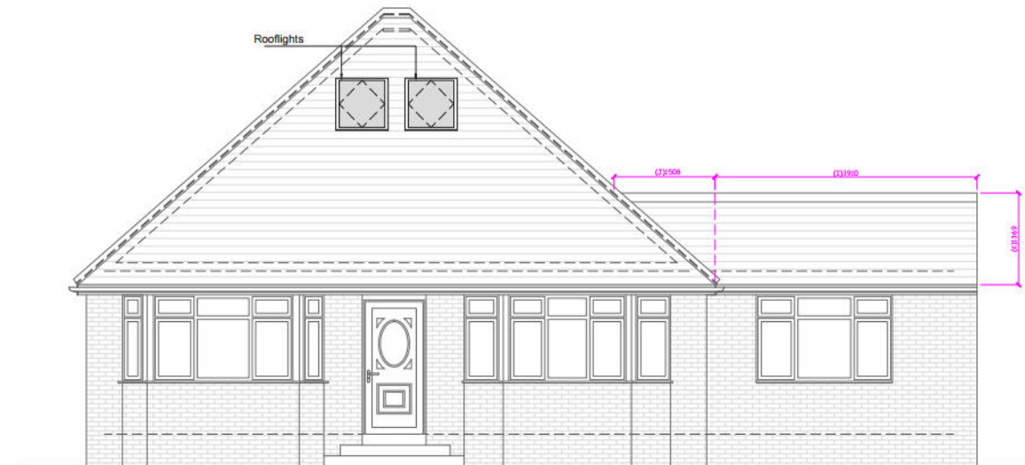
PROPOSED FRONT ELEVATION SCALE 1:100
