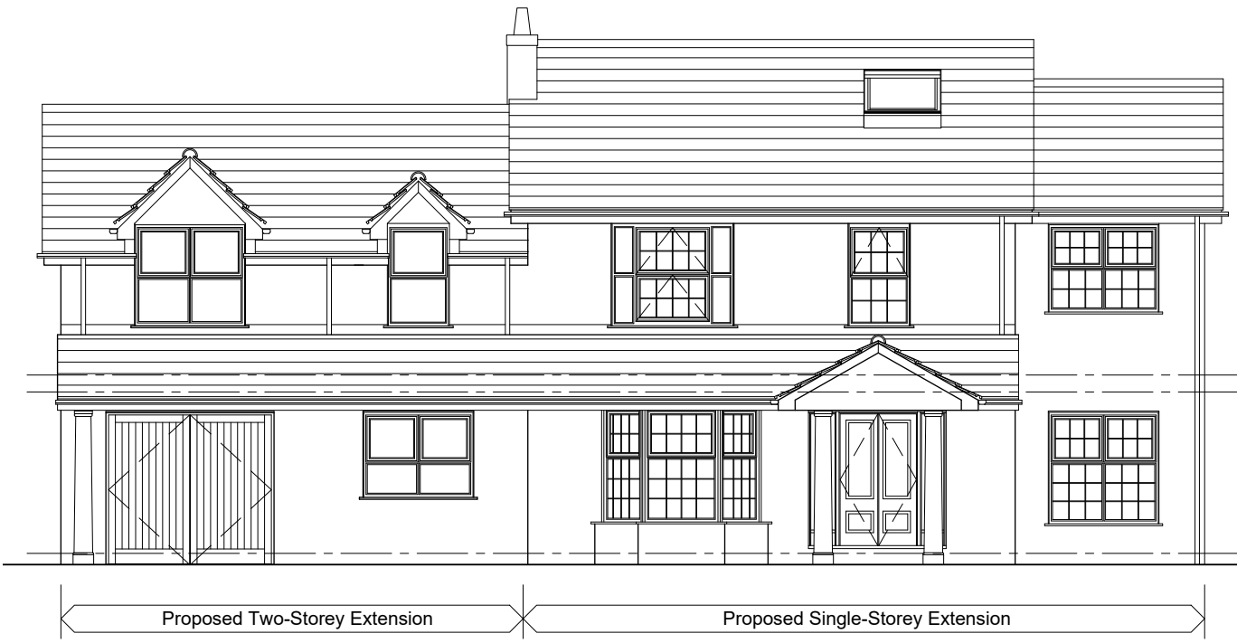
FRONT ELEVATION As Proposed Scale 1:100
