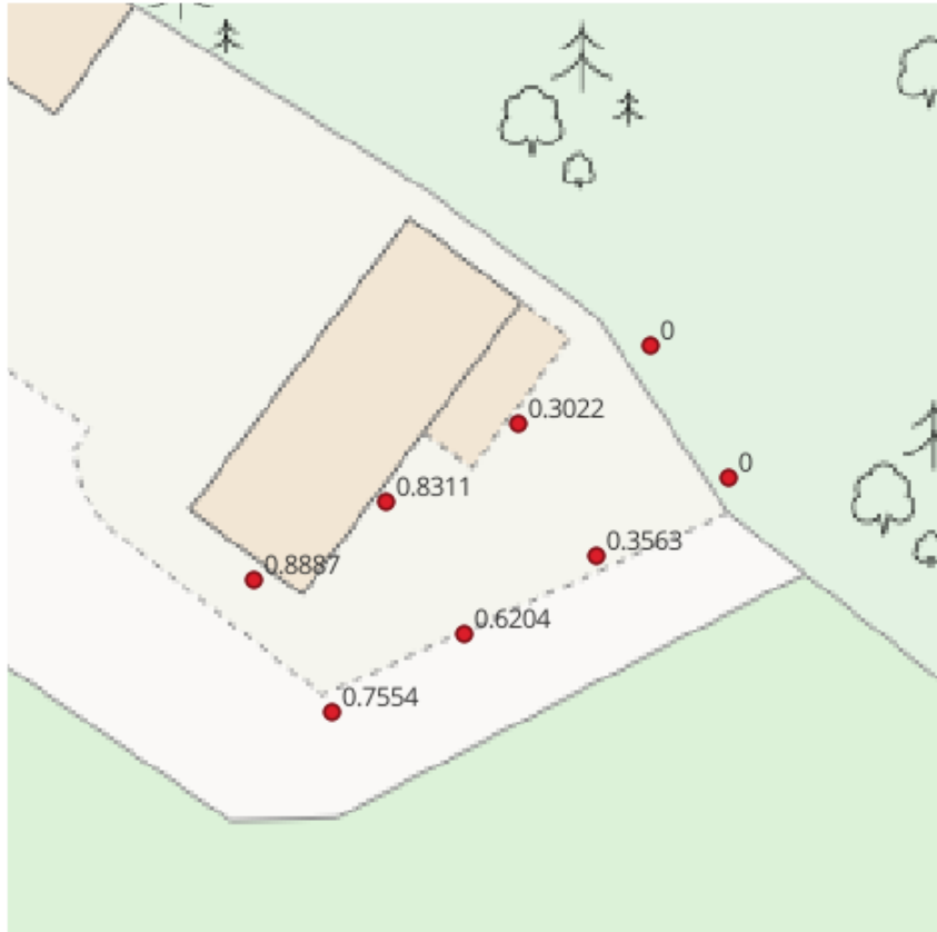
Figure 10: 1 in 100y+35% flood depths, m
