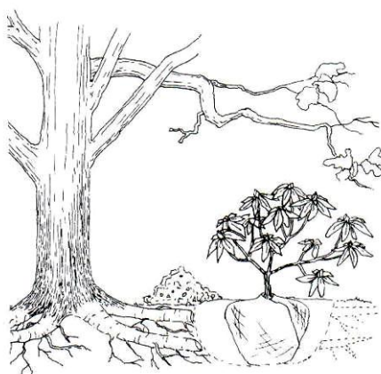
Figure 2: Root severance as a result of planting within RPA
