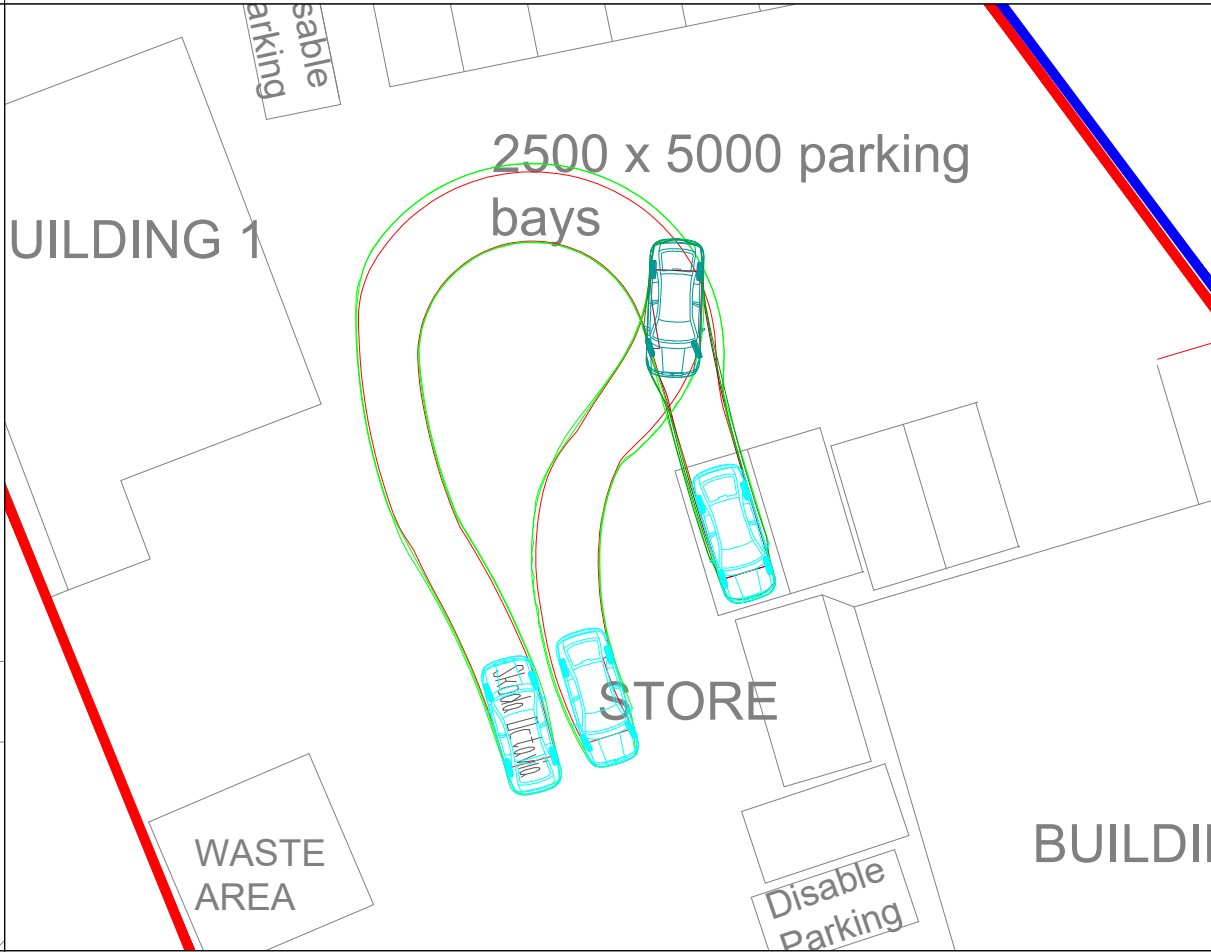
CAR PARK TRACKING 4
