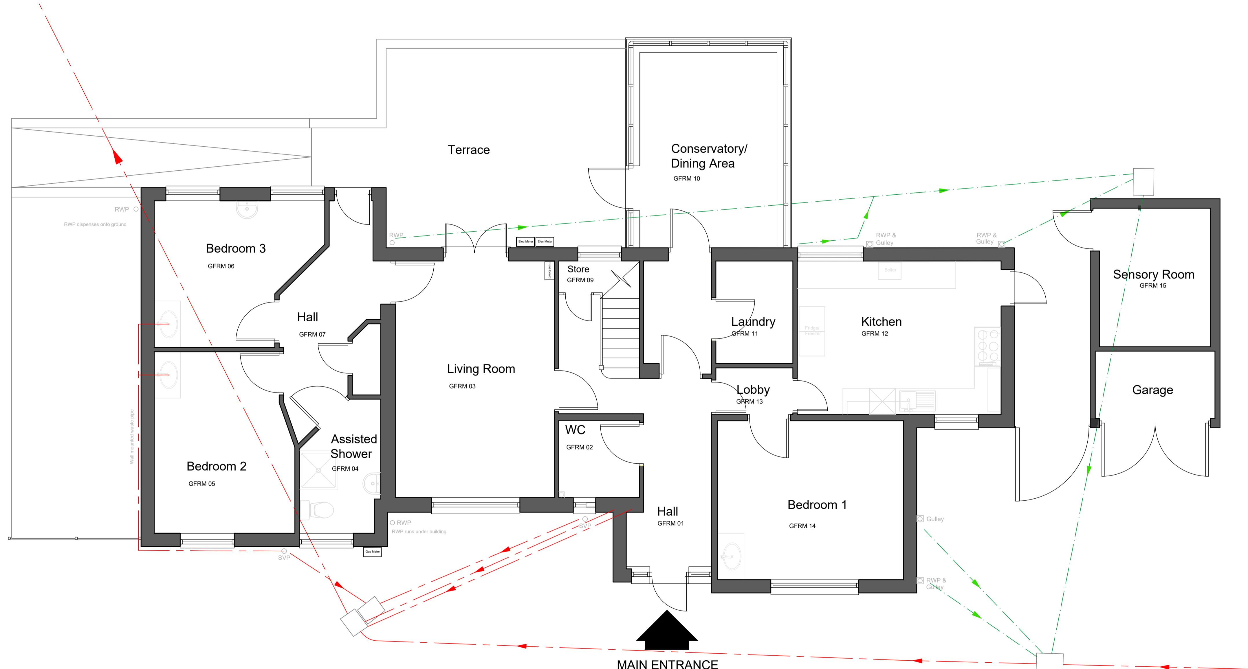
NOTE - Drainage layout shown is based upon Survey by Fosse Surveying. No building work to be undertaken within 3m of a Thames Water sewer without written consent.
